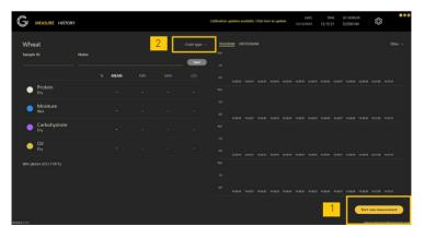
3) After you have started a measurement, a small pop-up screen appears telling you that a reference measurement is being taken and shortly after that the device is ready for a measurement and you can pour in the sample vessel (extra delay period can be adjusted, or null fired in the settings).
