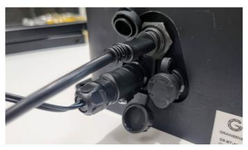
Please make sure to connect the power cable to the upper connector, which is designated for the power supply.
