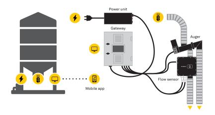
Via a grain entry and exit pipe system, grain is constantly flowing through the GrainSense Flow® sensor, where real-time analysis is performed. The measurement data is sent to the GrainSense Cloud, enabling the farmer to monitor the measured results in real-time and to make better decisions.
